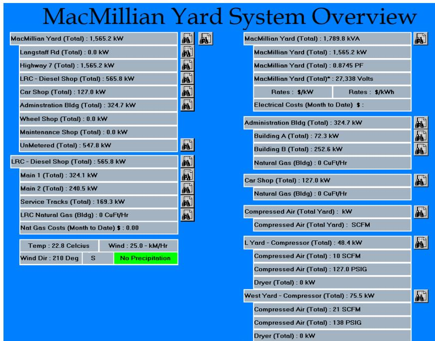
Figure 1 Example of a typical HMI Screen captured from the legacy PC-Based EMIS tool
