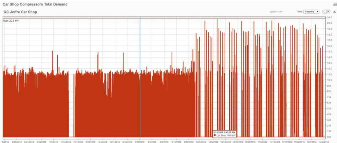
Figure 6 Compressed Air low-cost ECM results driven by EMIS insights. The figure shows the daily demand profile change.
