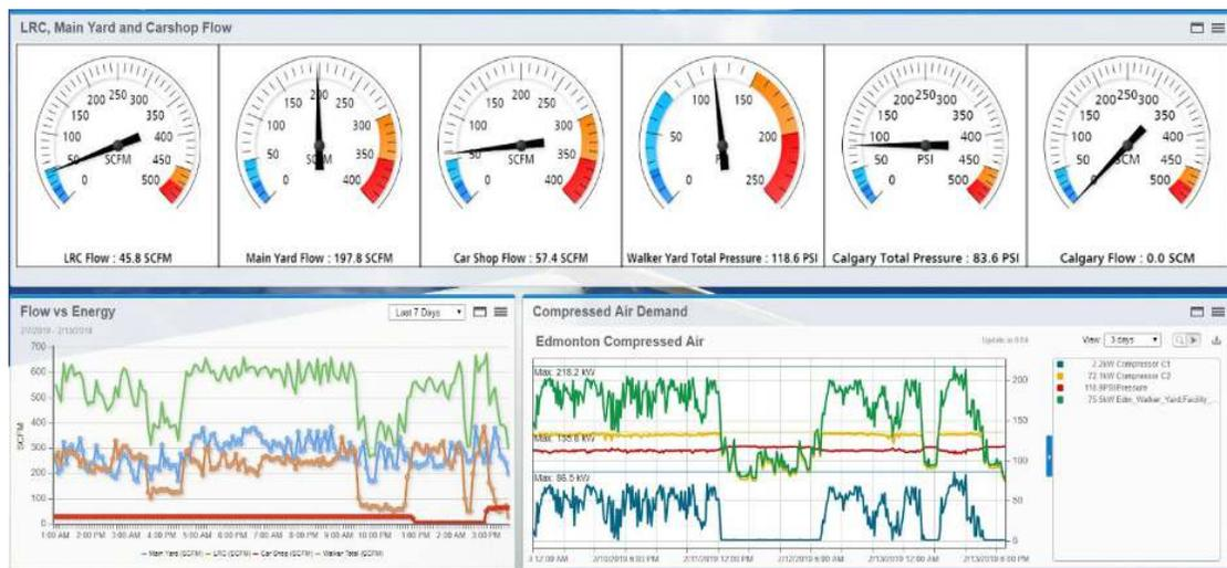
Figure 5 Compressed air monitoring example show flow, pressure, energy and demand in real-time.
