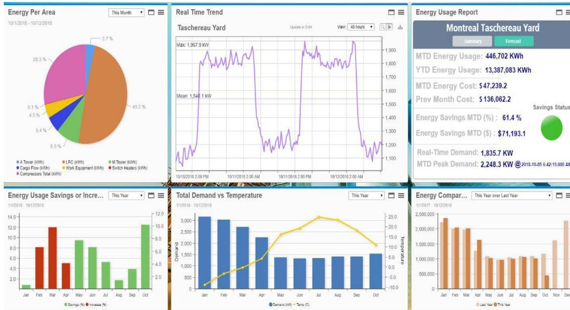
Figure 4 New main EMX dashboard for a typical large yard after the third iteration of feedback.
