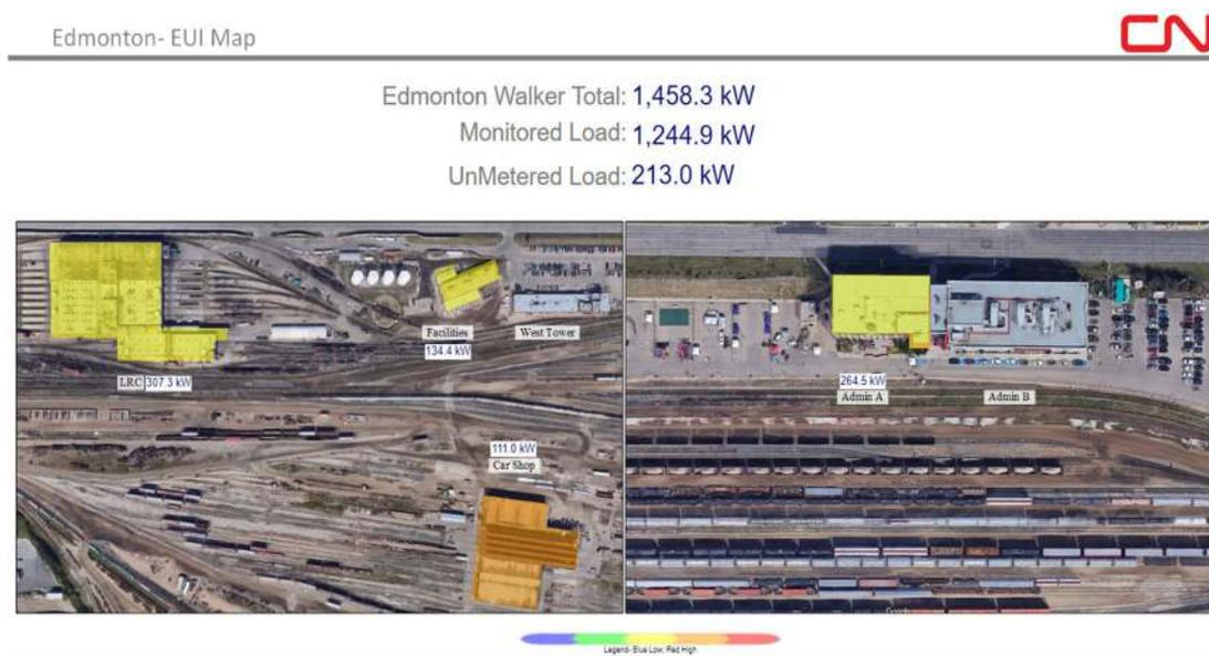
Figure 10 Pilot EUI Map visualization at a typical large yard.
