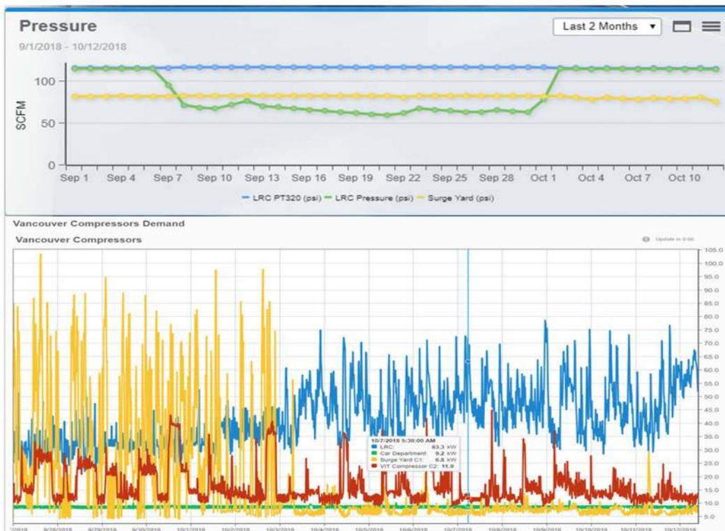
Figure 8 Compressed air close valve incident showing a drop in pressure throughout the incident period from the main line. The second graph shows the abnormal increase in power demand from the backup compressor.
